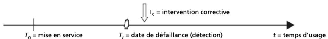
Figure 7 : Maintenance corrective
