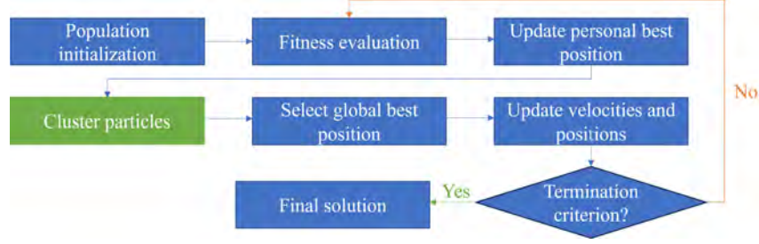
Figure 3.6: The flowchart of the hybrid EMOPSOC algorithm : MOPSO + ML clustering technique
