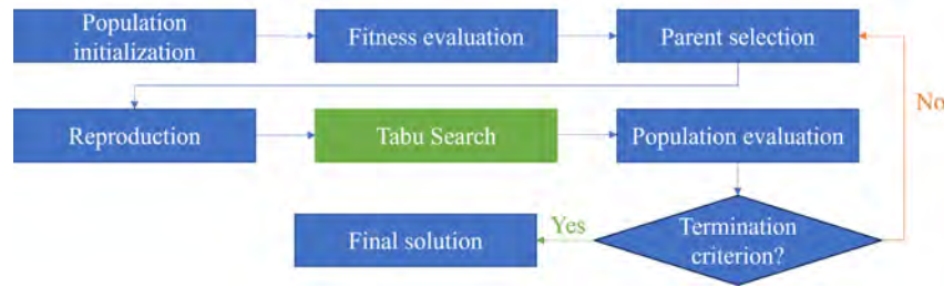
Figure 3.5: The flowchart of the hybrid algorithm: a genetic algorithm + tabu search
