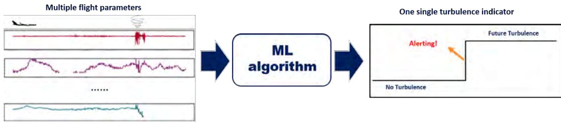
Figure 1.3: The machine learning based turbulence alerting function transforms on-board sensor signals into a turbulence indicator.
