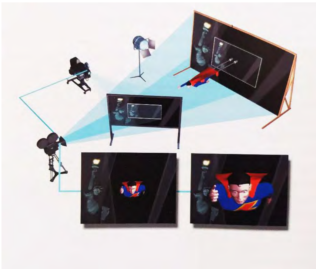
Figure IV-2 – Schéma du procédé Zoptic © Richard RICKITT, Special effects, the history and technique , London : Billboard Books, 2000, p. 70.
