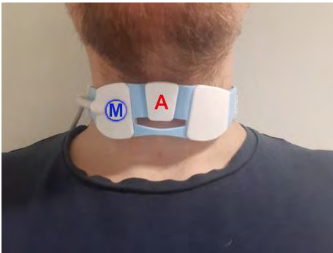
Fig. 2 Illustration of the Swallis DSA™ device. Cervical positioning of the Swallis DSA™ collar on a subject's neck. M: Microphone; A: Accelerometer (not used for this study)
