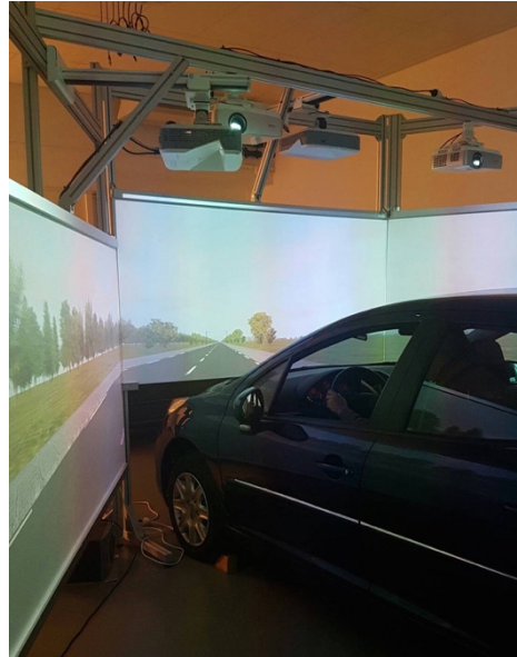
Fig. 1. The OKTAL driving simulator on the SIMUL’AUTO platform, at Toulouse 2 Jean-Jaurès University. [In color]
