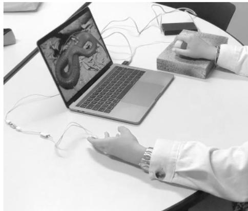
**Fig. 1** Experimental setup. The participant looks at the screen and squeezes the stress ball while his\her EDA is recorded by the BITalino sensor.
